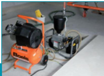
Membrane airless machine with compressor drive
