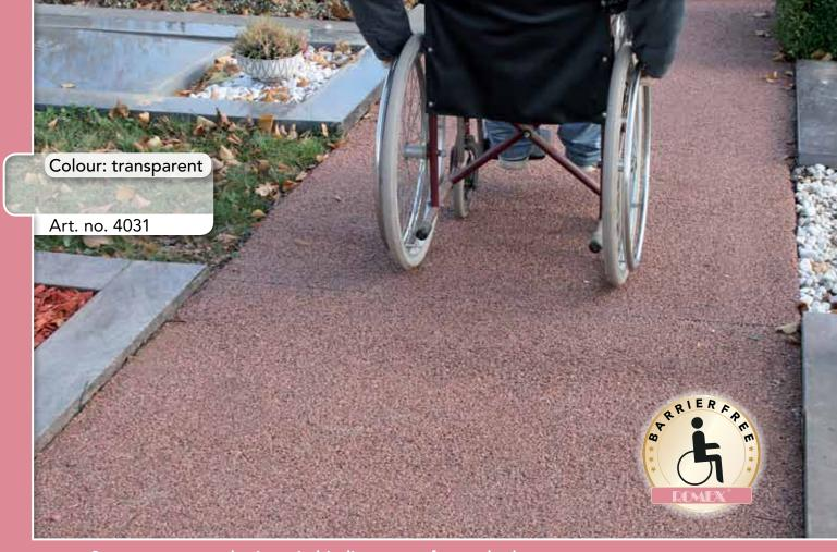
2 component synthetic resin binding agent for washed, dried and dustfree gravel and grit (grainsize from approx. 2 - 10 mm).\*1
